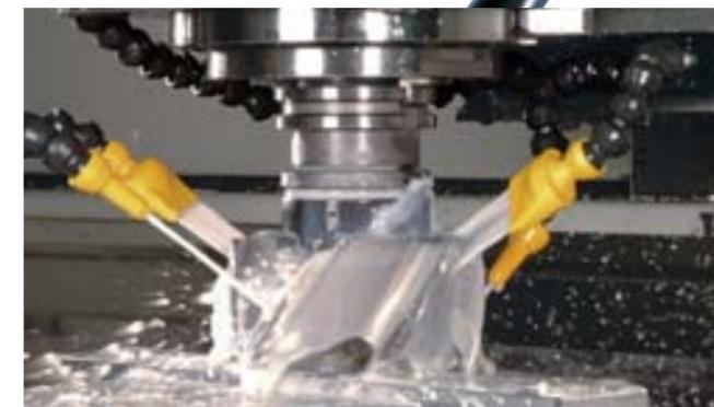
The Wiha maxiflex® universal articulated hose system is dimensionally stable, individually adjustable and has a long service life.
