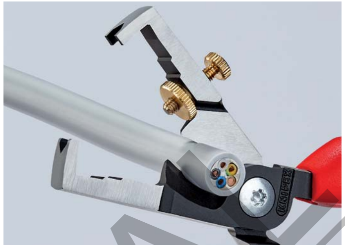
Induction hardened shear blade with precisely ground cutting edges for crushing-free cutting of copper cables up to Ø 15 mm (5 x 2.5 mm 2 )
