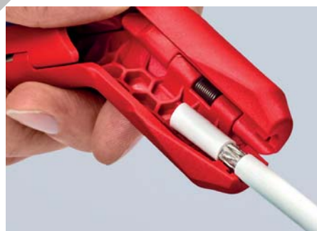
Stripping of a coax cable
